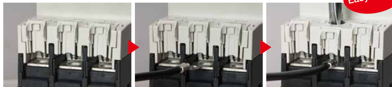
① Screw holder lifts up the screw. ② Insert a round solderless terminal ③ Tighten the screw
