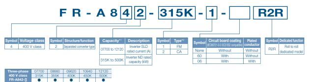
\*1 Models can be alternatively indicated with the inverter rated current (SLD rating).
