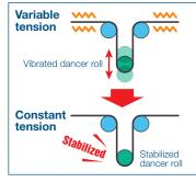
When material rupture (break) occurs and the sensor feedback value (dancer/tension feedback) is held at the upper/lower limit for a certain period of time, the break detection signal is output.
