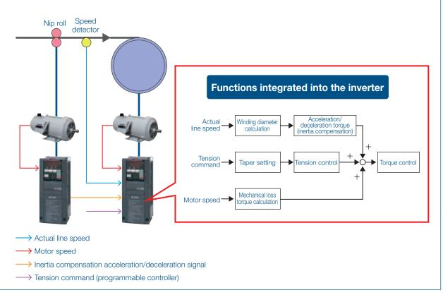
Example of tension sensorless torque control
