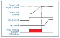
•The present winding diameter is calculated from the line speed and the actual motor speed. (The system must be started at low speed.)
